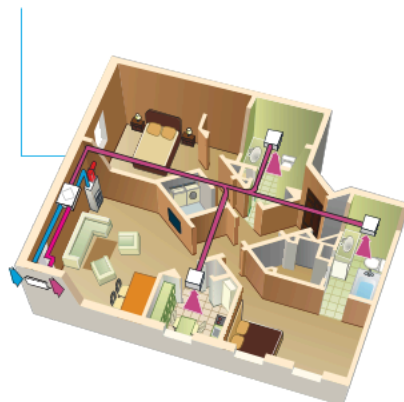
HRV with Fan Coil System
