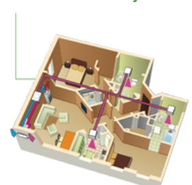
ERV with Fan Coil System
