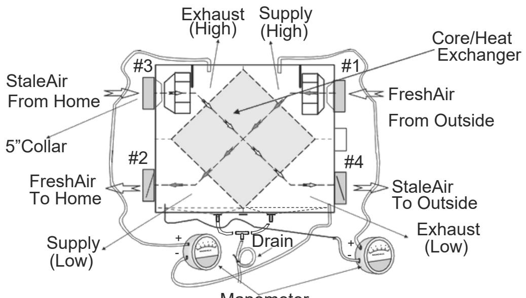
**NOTE:** Make sure to plug back all holes after balancing.
