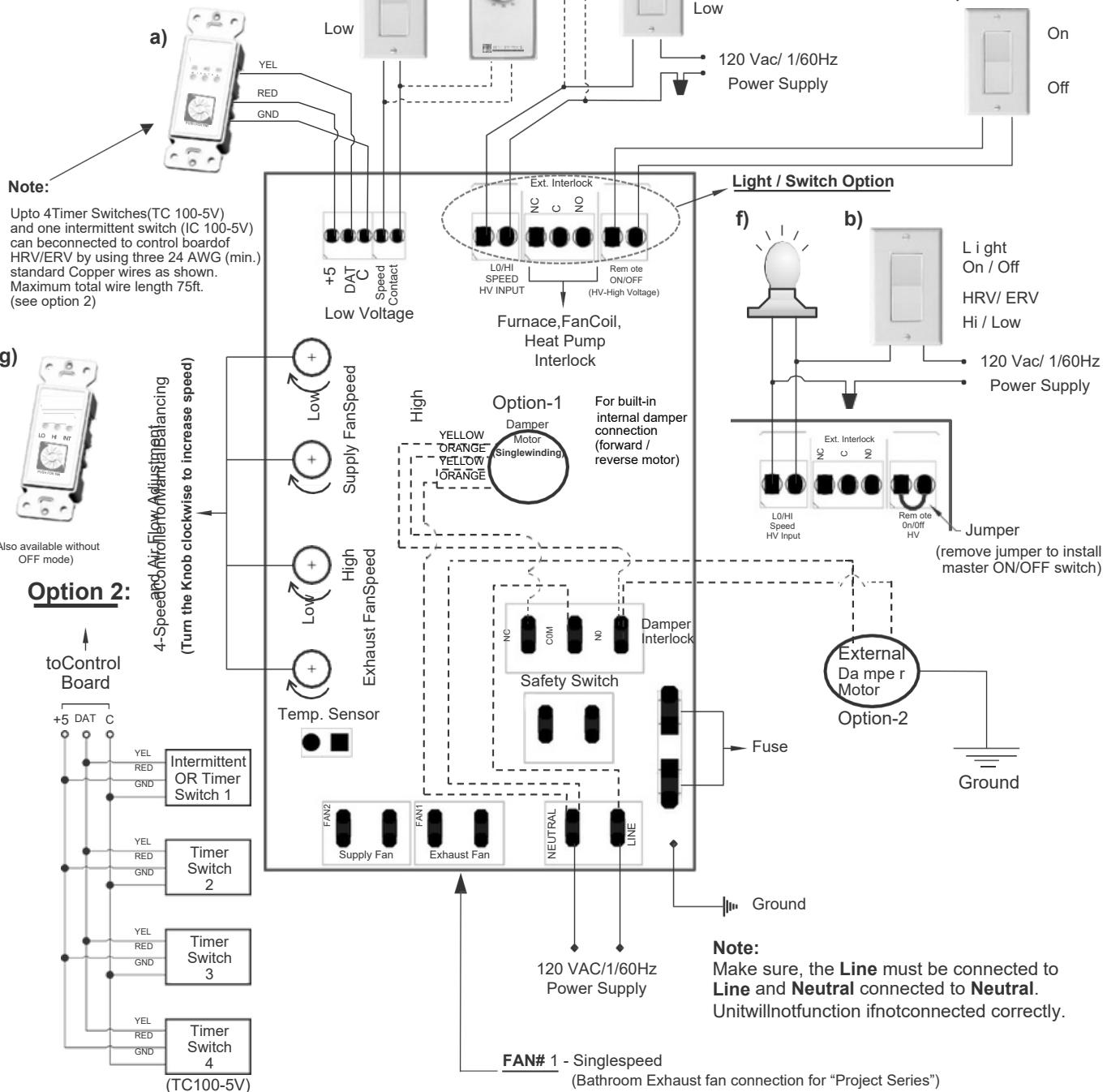
**Important Note:-** When installing timers or time delay switches, make sure that they are for appropriate HRV/ERV models.
